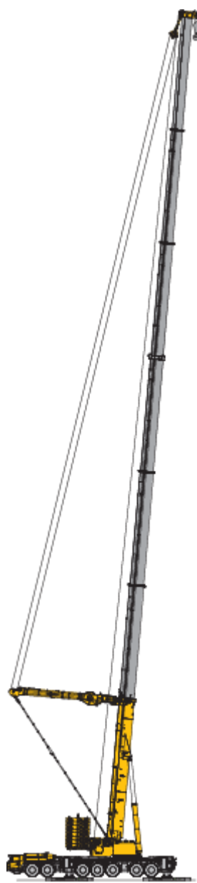
超起+主臂 Super lifting device + boom
